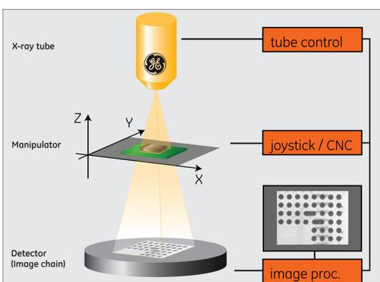
**Set-up** of a X-ray system with transmission tube, manipulator and vertical X-ray beam. The magnification is selected by adjusting the Z-position of the specimen. Processor based control units enable automated inspection cycles and image evaluation.
